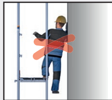
Pay careful attention to any possible risk of falling between the scaffold and the building
