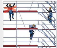
Only use fitted ladders or stairways for ascent and descent
