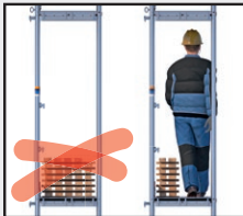
When material is stored, make sure there is still sufficient space left to move along the decking
